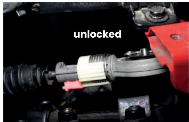
22.3 Hold the selector lever in the center position by a second person
