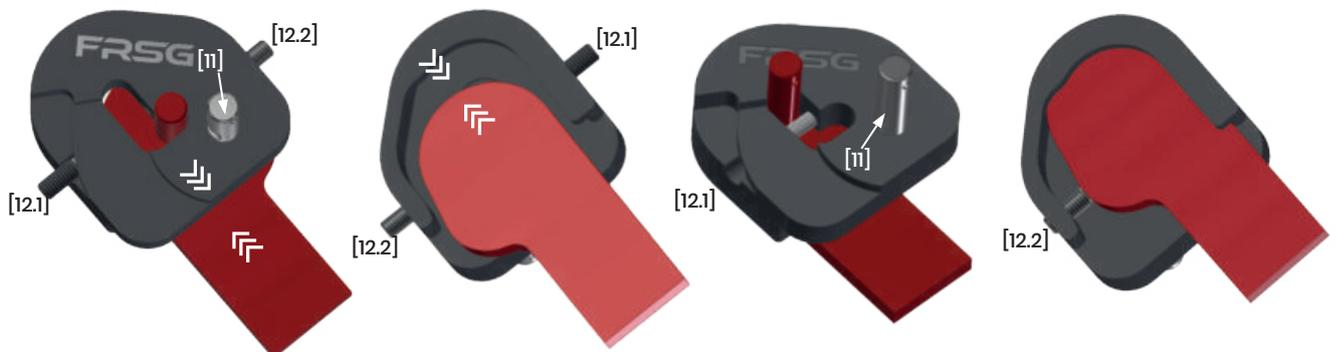
22. Check that all gears can be engaged without any problems and that the selector lever, in the interior of the vehicle, is in the center position
